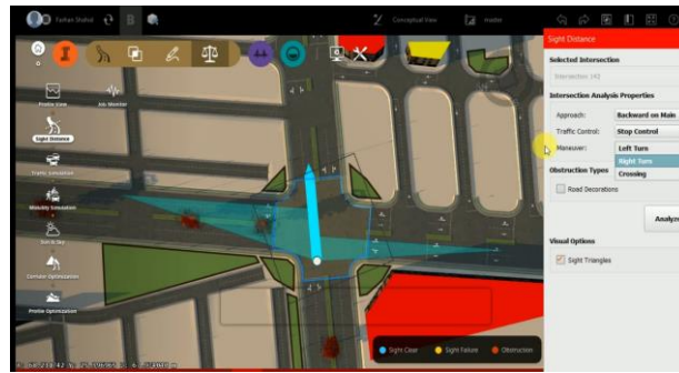
Fig. 4:Sight Distance Analysis on Road model (INFRAWORKS-360)
