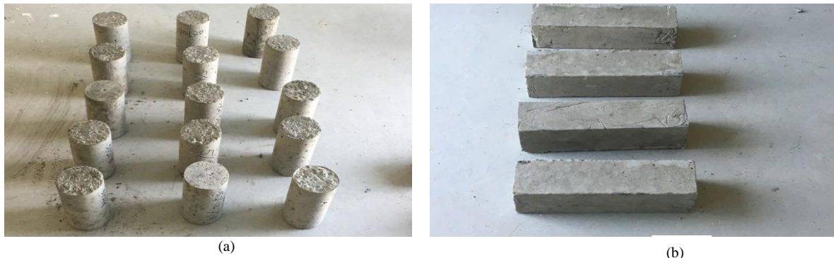
Fig. 1: Concrete test specimens used in the experimental program (a) cylinders (b) beams
