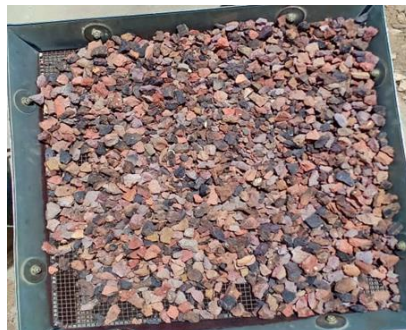
Fig 1: Crushed Over-burnt Bricks
