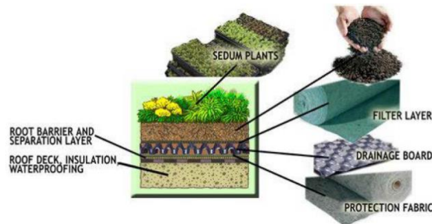
Fig. 2. Extensive roof's installation pattern
