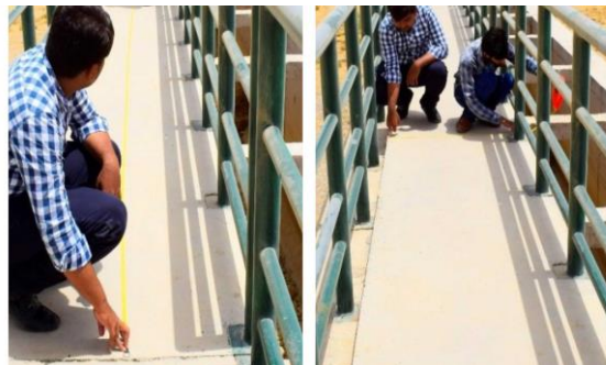
Fig. 5: Measurement of Length and Width of Aqueduct
