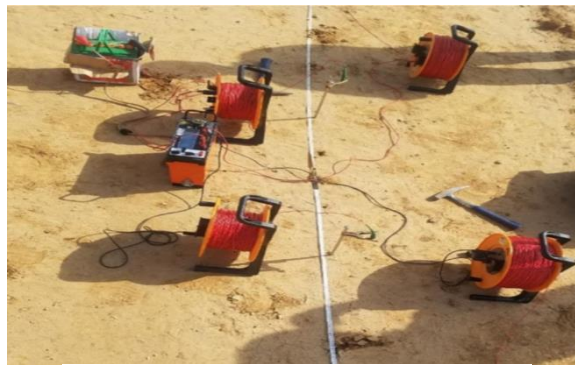
Figure 2 Terrameter with current and potential wires attached [14]
