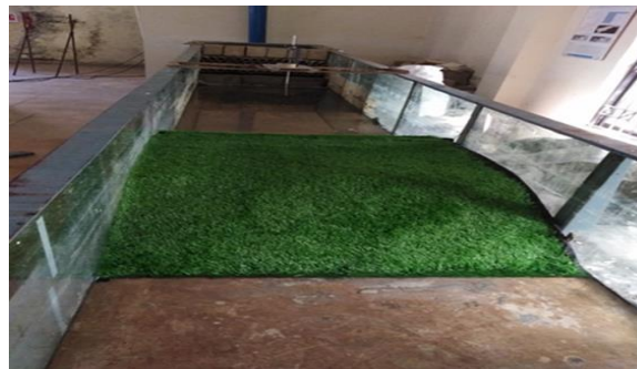
Fig. 2: Embankment Weir with Grass Vegetation
