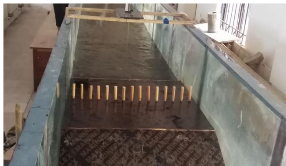
Fig. 4: Embankment Weir with Rigid Vegetation at the Center of Crest of the Weir
