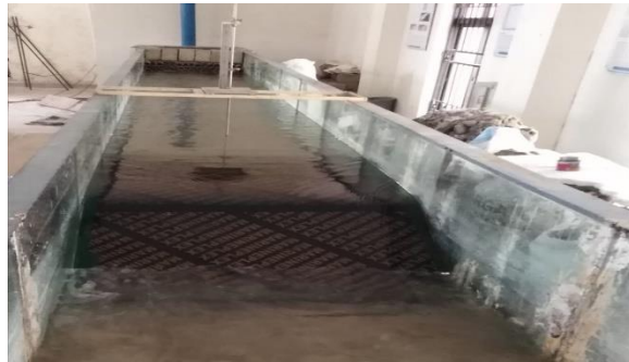
Fig 1: Smooth Embankment Weir
