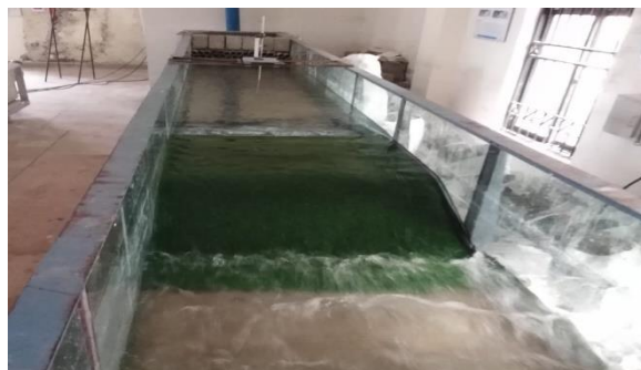
Fig. 2: Embankment Weir with Grass Vegetation
