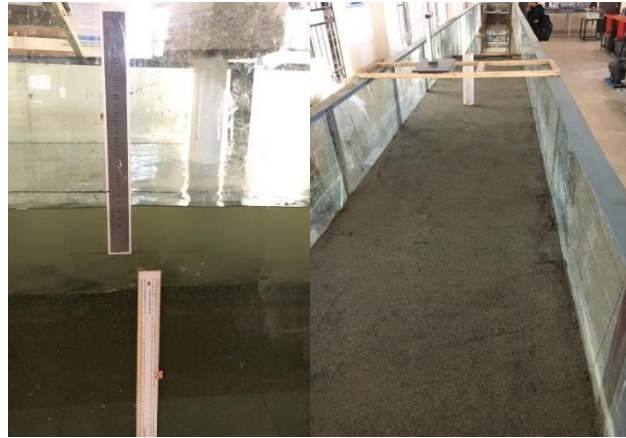
Fig. 6 (a) and (b): Flow depth kept equal to 13cm & Point gauge mounted on a levelled carriage.
