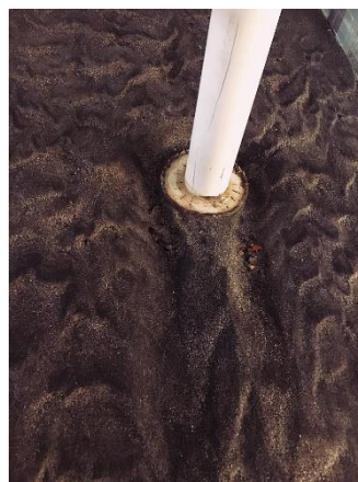
Fig. 9: Scour Pattern around compound pier in case R2.
