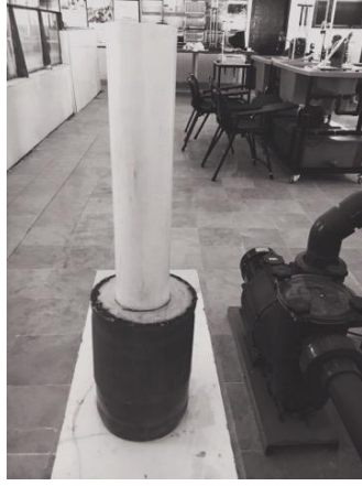
Fig. 4: Definition diagram and pictorial view of circular compound pier used in the experiment.
