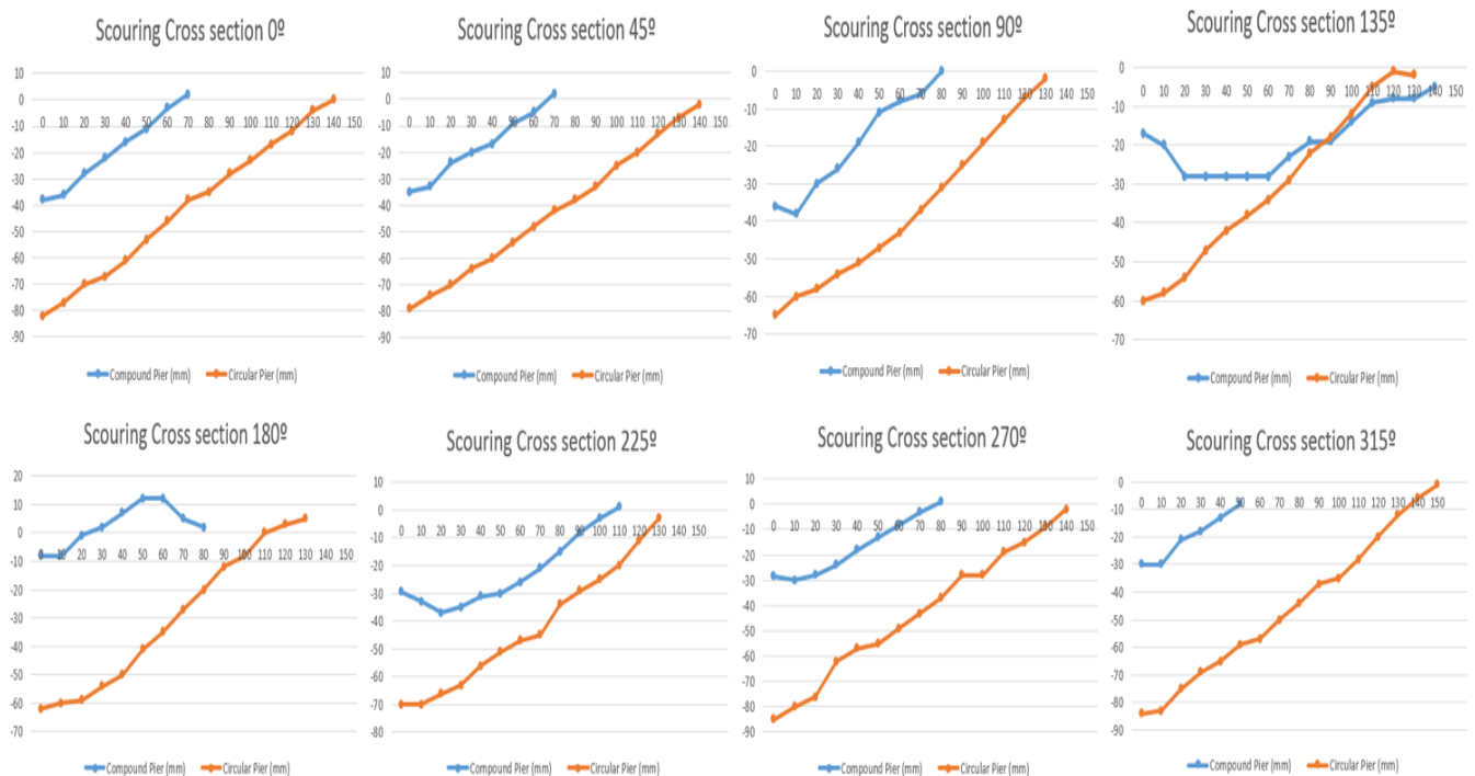
Fig. 10: Effect of circular and compound piers on longitudinal and lateral profiles.
