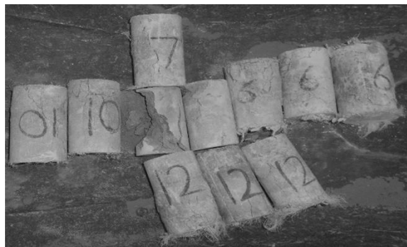
Fig.5: Simulation of Cracks after Compression
