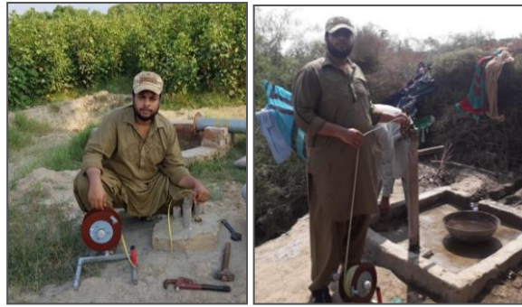
Fig.5: Water level readings collecting from Piezometer and hand-pump at command area of Muhammad Khan distributary
