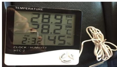
Fig. 7. Device used to measure indoor and outdoor temperature
